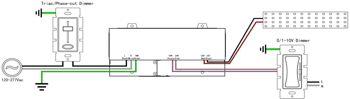
1. Input cable 3\*18AWG, the Green cable to GND, Black cable to L, and White cable to N of Mains AC.
